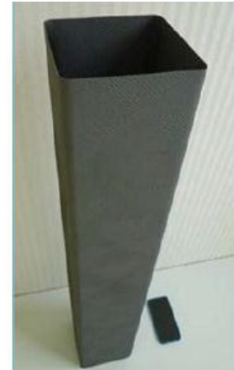
132.5mm×800mmL Channel Box ( \text{SiC}_f\text{-SiC} )
