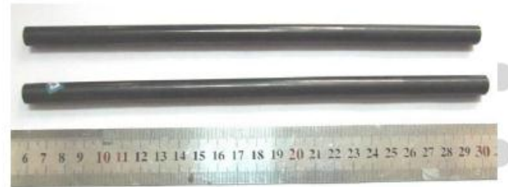
■ SiC/SiC f composite tube
