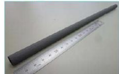
Φ10mm×280mmL Cladding Tube ( \text{SiC}_f\text{-SiC} )
