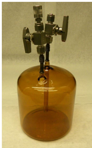
Figure 3.11. Irradiation vessel for gas phase experiments
