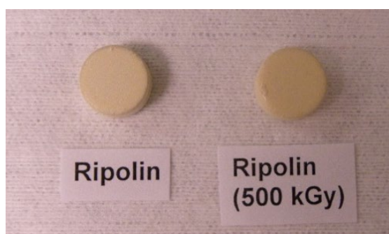
Figure 3.3. Ripolin coupons before and after irradiation
