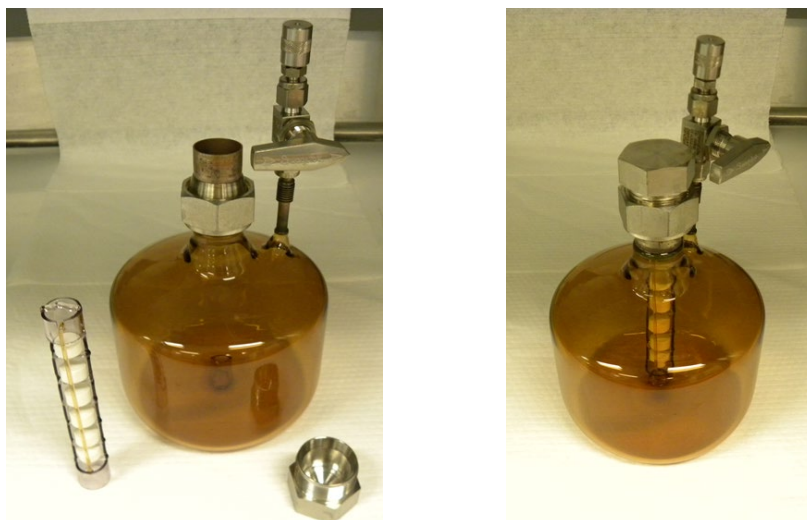
Figure 3.10. Photographs of the new O-ring free irradiation vessel and coupon holder design, with components disassembled (left) and fully assembled (right)
