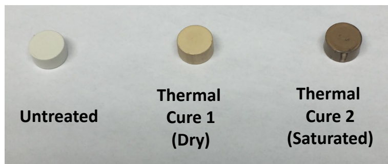
Figure 3.2. Coupons before and after the thermal cure processes
