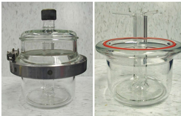
Figure 3.7. Irradiation vessel (shown pre-irradiation and without the coupon holders)
