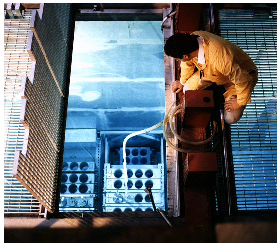
Figure 1. Low intensity cobalt array facility for radiation and thermal ageing
