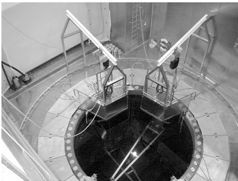
Picture 3. Picture of the two work shafts attached to the flange of the reactor pressure vessel
