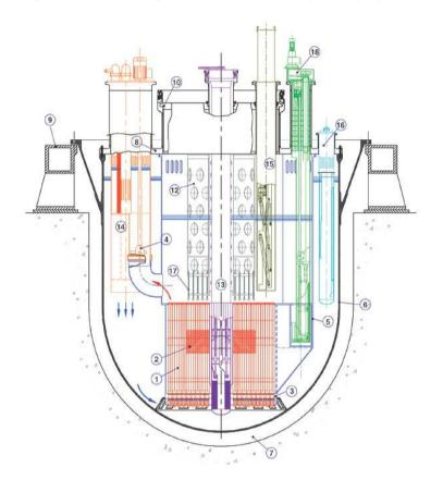
Figure 13: EFIT design and scheme of the primary system
