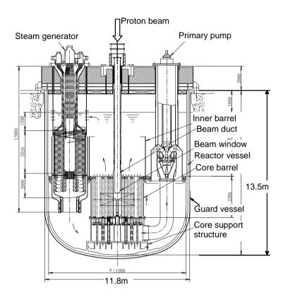
Figure 10: Conceptual design of JAEA's reference ADS
