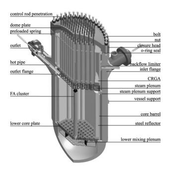
Table 17 reports some design characteristics of the RPV and internals of the HPLWR [3]. These operational conditions are based on the design data of Oka for in-core components and the design recommendations of Bittermann for the RPV [4]. The HPLWR has a modified core assembly in order to use fuel with lower enrichment, has its hot steam completely separated from the RPV and includes several safety features added to the original Oka design [5].
