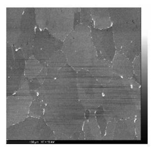
Note: The light contrast at the grain boundaries correspond to tungsten precipitates.
