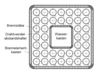
Brennstäbe = fuel rods; Drahtwendelabstandshalter = wired fuel rod spacer; Brennkasten = fuel assembly box; Wasserkasten = water (moderator) box.
