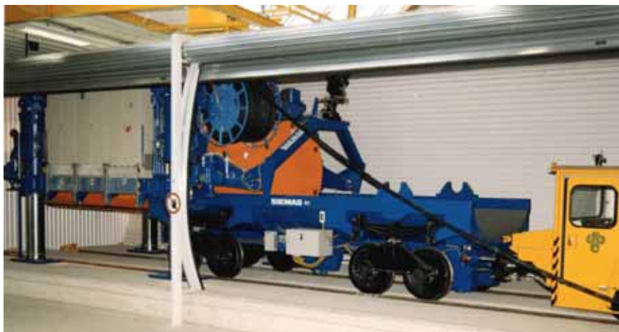
Figure 2: Emplacement of a POLLUX cask in a drift
