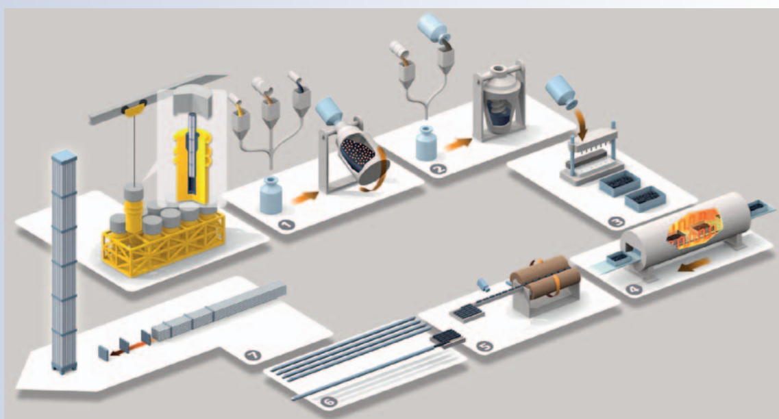
Figure 8: MOX fuel fabrication
