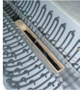
The STEM Project: The START test facility (left) and the alumina crucible (right) with RuO 2 powder in the quartz tube.
