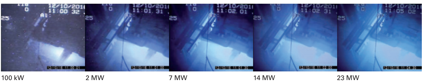
Photos looking down into the reactor pool showing the Cherenkov radiation characteristic of the different core powers. IRSN, France
