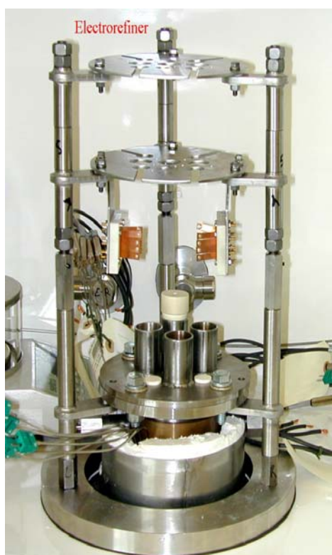
Figure 8.10: Photograph of NNL electrorefiner for Pu-U-Am electrorecovery and partitioning from Nd and U
