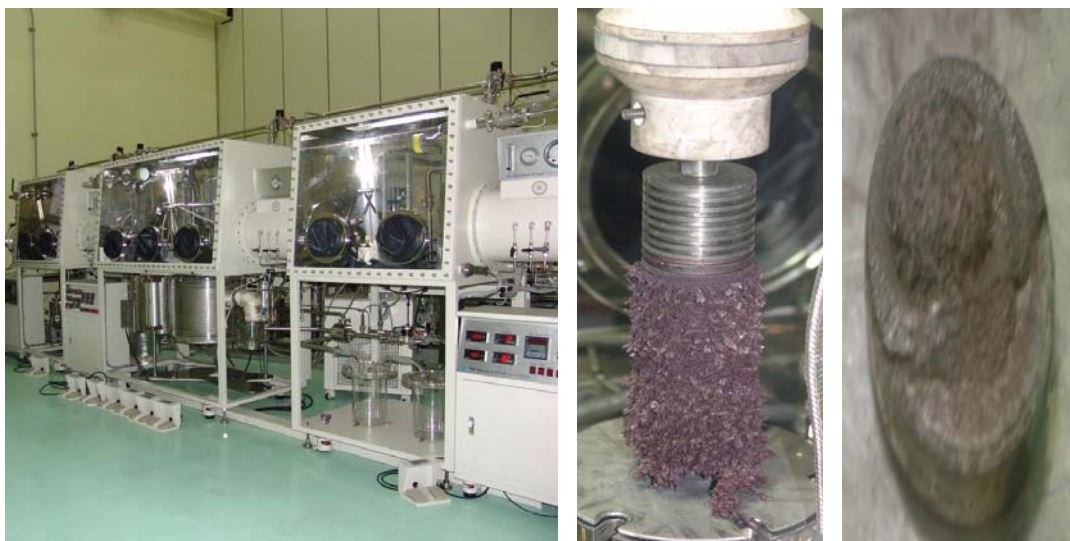
Figure 5.6: Electrorefiner system (left) and the received uranium dendrite (middle) and uranium ingot (right)
