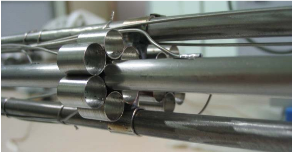
Figure 2.6 – Picture of the NACIE spacer grid (before operation)
