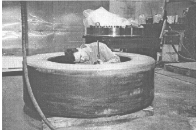
Figure 5. Ring-shaped block for surrounding a canister (Clay Technology AB). Weight about 2 tons, diameter 1.75 m and height 0.4 m. The block was made by uniaxial compaction under 100 MPa pressure
