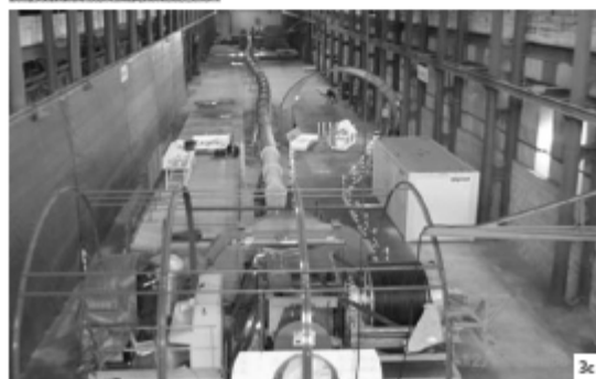
Fig. 3a & 3b: Bentonite rings removal test in view of waste package retrieval in Sweden (Åspö HRL, 2006) Fig. 3c: Retrieval of a disposal HLW package from a simulated emplacement cell in France (ESDRED programme, 2008)
