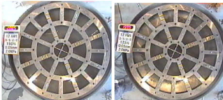
Plate 2: Complete penetration of grout Plate 3: Limited infilling of the model fracture through the model fracture
