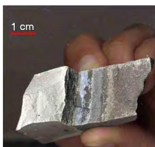
Figure 1: Observation of a centimetric perturbation front within the argillite after 15 years of argillite/concrete interactions (Tinseau, personal communication)
