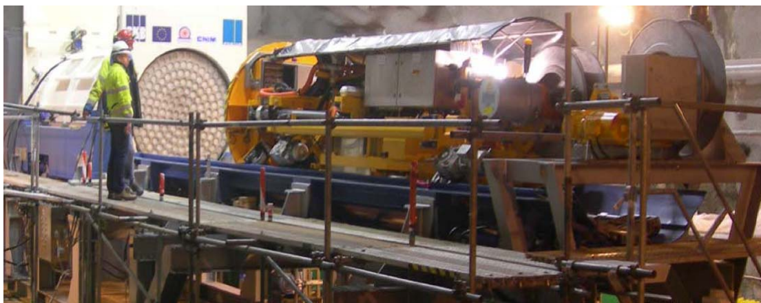
The KBS-3H supercontainer and emplacement machine (Sweden)
