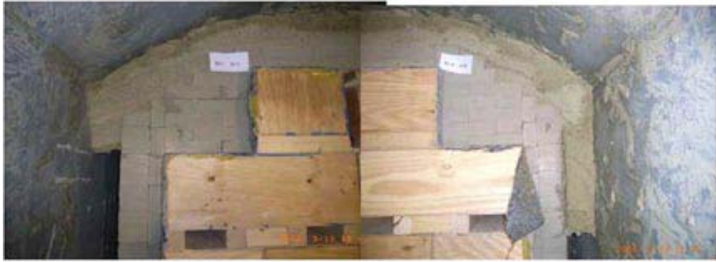
Figure 3.8 Large-scale testing of water uptake by backfill emplaced according to SKB's current concept involving bentonite blocks and pellets (SKB 2008b).
