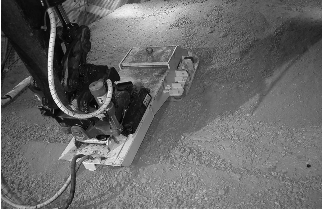
Figure 7. Test of granular backfill emplacement by the previous concept in the Swedish underground laboratory at Aspo
