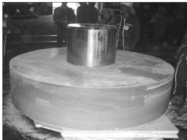
Figure 2-5. The first clay buffer ring during stripping
