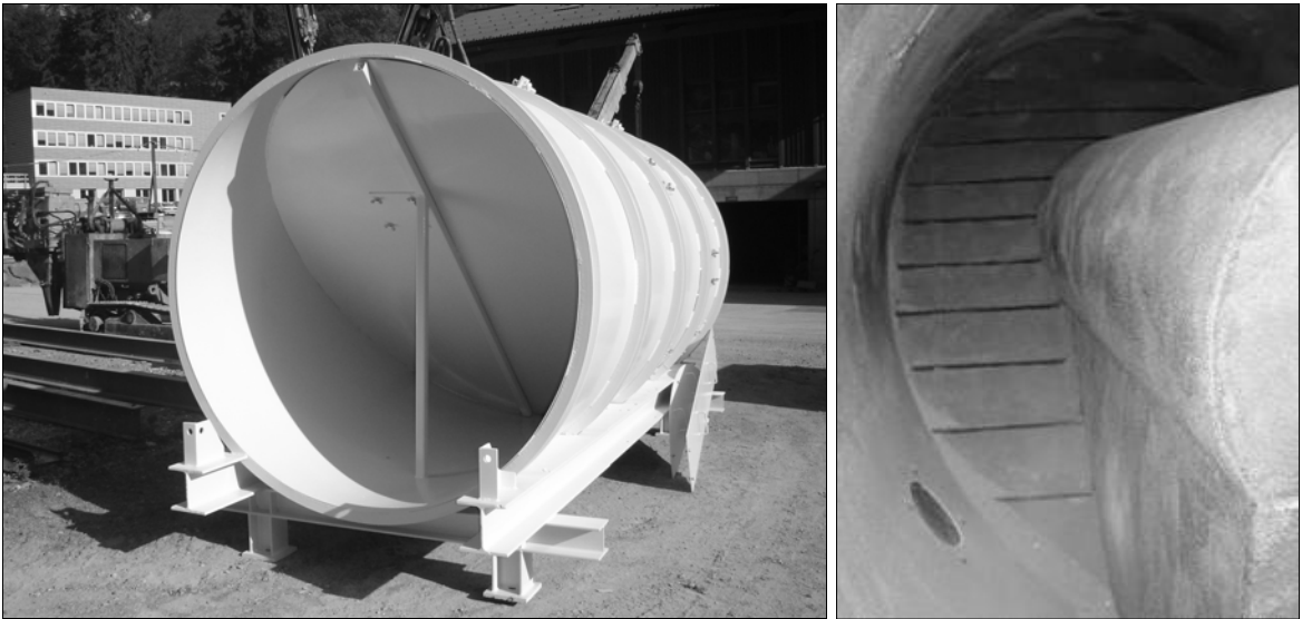
Figure 4-4: Photos of the steel model for the planned emplacement tests for buffer
