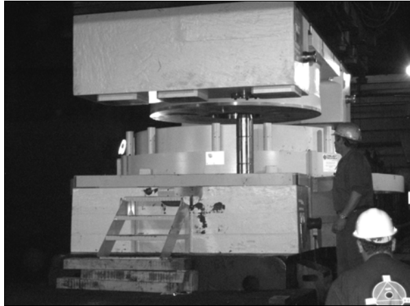
Figure 2-3. The mould before pressing the first ring
