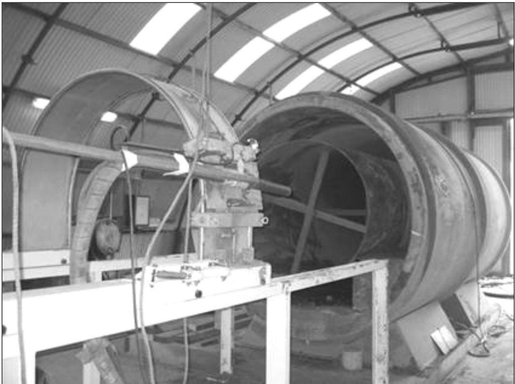
Figure 3-3. 2/3 rd scale mockup for the testing of dry granular backfill (situation in June 2006)
