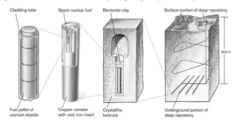
Figure 1. The Swedish KBS 3 concept for geologic deposition of spent nuclear fuel
