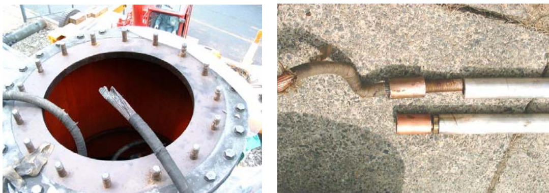
Figure 0-8: Photographs of the damaged lead wire and shield plate of outer casing of transformer
