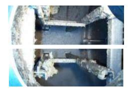
Fig. 2: Mineral wool specimen (left) and debris of fragments after a BWR-LOCA (right).
