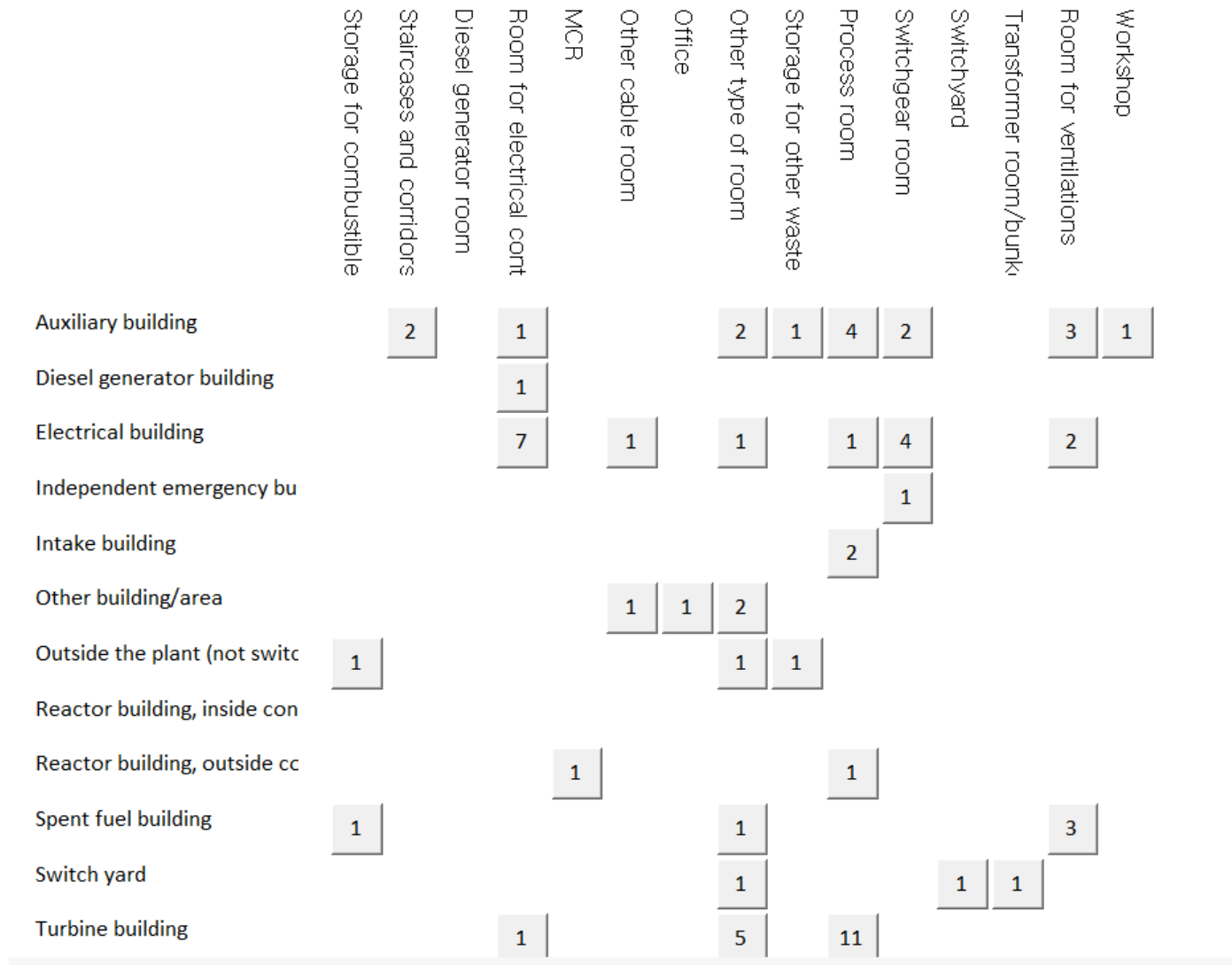
Figure 8. Number of fire occurrences in buildings/compartments for PWR at power operation with known average compartment numbers from countries reporting all events (screenshot from the OECD FIRE Database [3])
