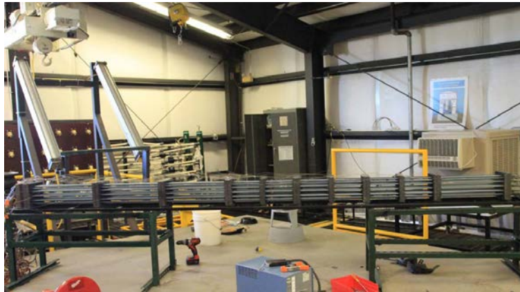
Figure 50: Single fuel assembly for Phase 1 PWR testing in construction stage.
