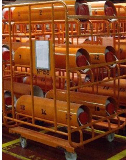
Figure 3: Tubular carriage for the transfer of drums
