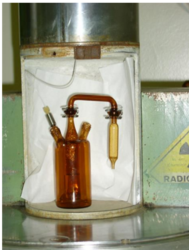
Figure 1. The reaction vessel shown within the irradiation chamber of PSI's \gamma -irradiation cell.
