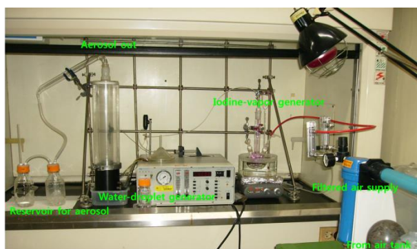
Fig. 1. Photo of lab scale set-up for a behavioral study of volatile I_2 from water droplets-air flow.
