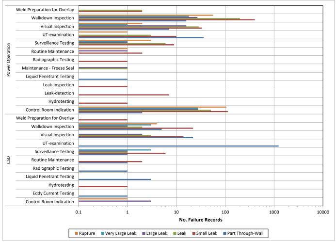
Figure 6: Non-code pipe failures by plant operational state and method of flaw detection
