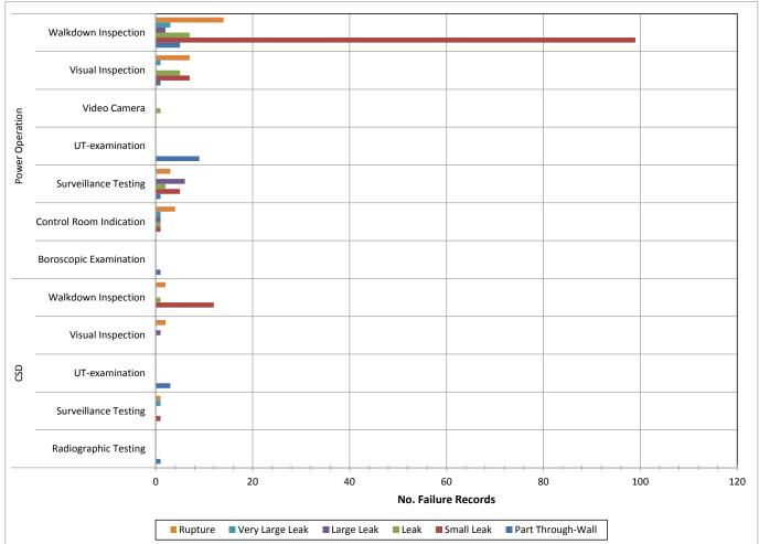
Figure 7: Fire protection water system pipe failures by plant operational state and method of flaw detection
