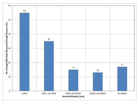
Figure 13: Through-wall class 1 pipe flaws discovered through pressure test
