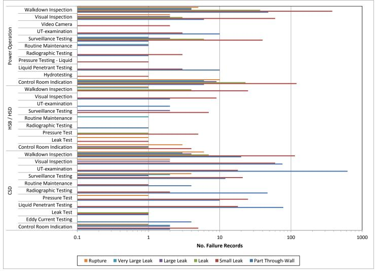
Figure 4: Code class 2 pipe failures by plant operational state and method of flaw detection
