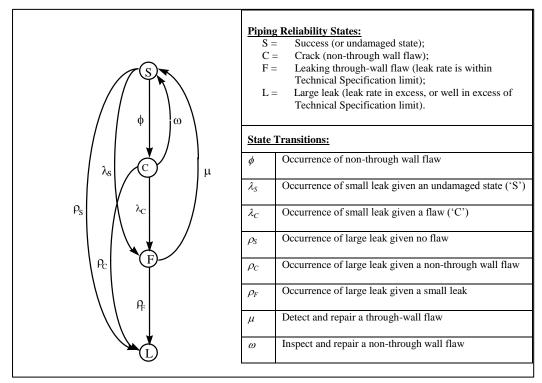
Figure 14: Markov model of piping reliability
