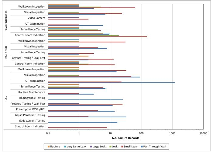
Figure 3: Code class 1 pipe failures by plant operational state and method of flaw detection<sup>1</sup>
