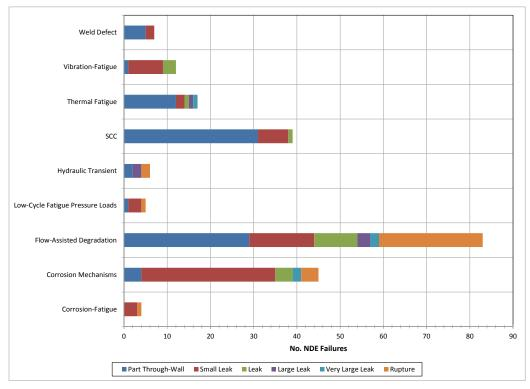
Figure 12: LTA-RIM by failure mechanism and failure mode
