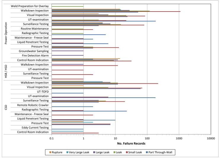
Figure 5: Code class 3 pipe failures by plant operational state and method of flaw detection
