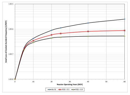
Figure 15: Influence of POD on structural integrity<sup>3</sup>
