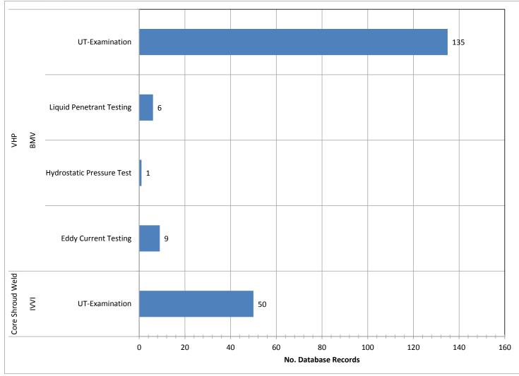
Figure 8: Core shroud weld cracks and vessel head penetration cracks by inspection method and technique
