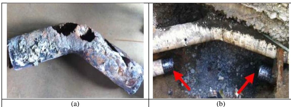
Figure 21: a) Corroded Elbow, b) Leak Area Wall Thickness Measurement, c) Underground Buried Pipe Coupling Connection, d) Anti-Corrosion Tape
