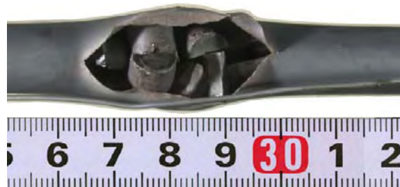
Figure 7.37 Through wall cracks with brittle appearance. Halden IFA-650.2 test
