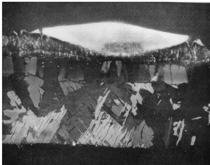
Figure 6.22 High-temperature oxidation below an oxide nodule formed during pre-oxidation 80×
