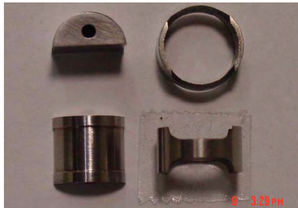
Figure 5.15 Components of a ring tensile test, D grip to the left and specimen to the right [29]
