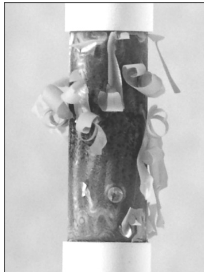
Figure 6.70 Specimen of E110 cladding that exhibited severe breakaway oxidation after 1 400 seconds at 1 000°C
