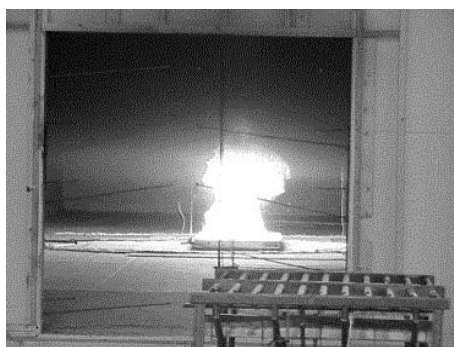
Figure 1: Photograph of a 1 MW heptane fire seen through the open doorway
