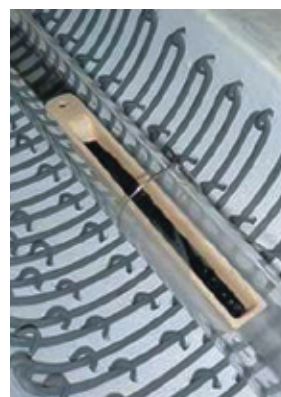
The STEM Project: The START test facility (right) and the alumina crucible (left) with RuO 2 powder in the quartz tube. IRSN, France
