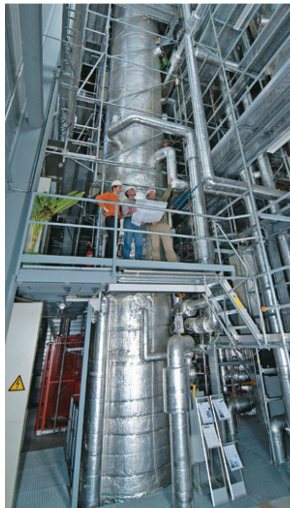
The PANDA reactor pressure vessel. Paul Scherrer Institute, Switzerland
