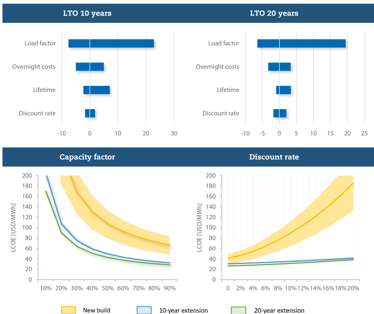
Figure 6.6: Sensitivity analysis of the LCOE of new build, and LTO of nuclear power plants
