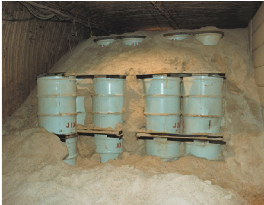
Figure 4.11: Typical intermediate-level radioactive waste emplacement
