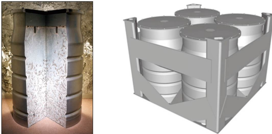
Figure 4.8: In-package grouted wasteform in a 500-litre drum (left) and the disposal unit (right)
