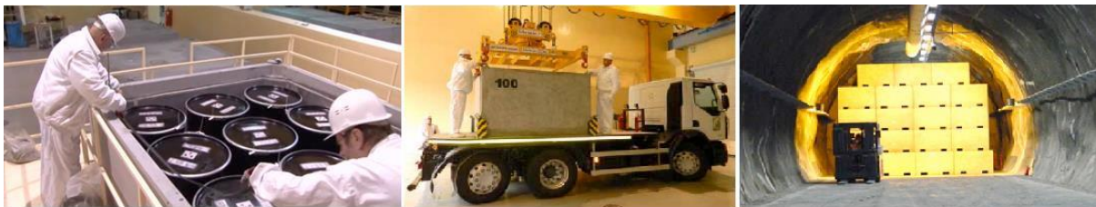
Figure 4.7: Steps towards the final disposal of waste in the NRWR (emplacement of drums in concrete containers, transportation and final disposal)
