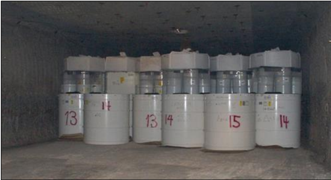
Figure 4.2: Supersacks of MgO emplaced on top of WIPP waste
