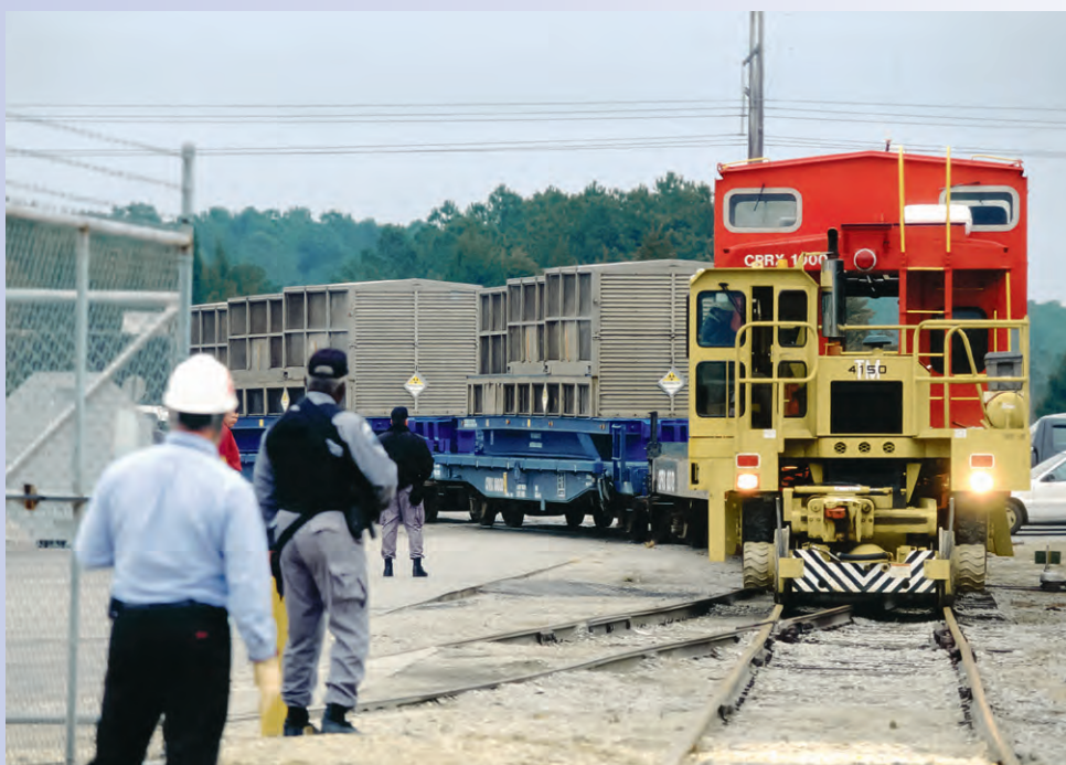
A rail transportation of spent fuel casks.
