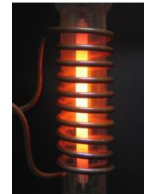
Inductively heated single-rod test
