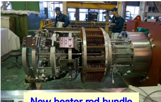
New heater rod bundle
