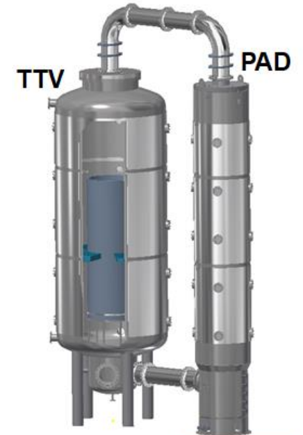
TTV: THAI test vessel PAD: Parallel Attachable Drum
