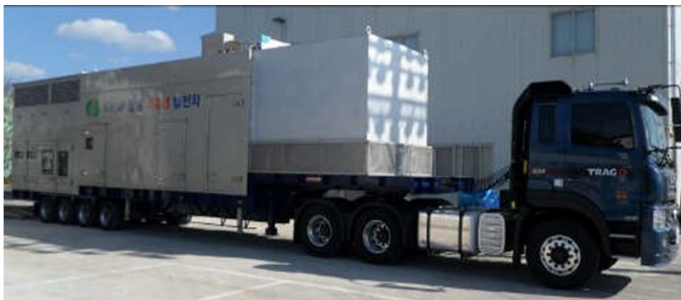
Figure 10. 3.2 MW mobile diesel generator (Korea)
