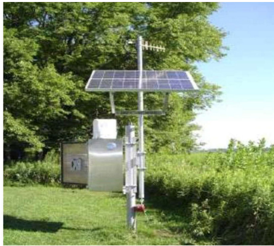
Figure 2. Remote Automated Gamma Monitoring Station
