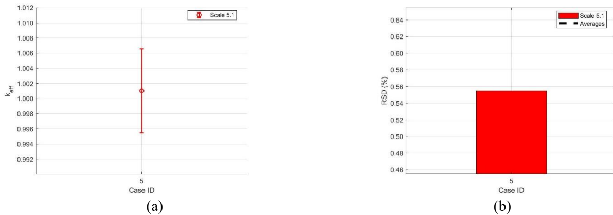
Figure 3.50. Calculated k -inf for I-3 VVER-KOZ-6 full core at HZP: (a) mean value with uncertainties, (b) RSD grouped by covariance libraries utilised
