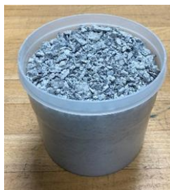
Figure 3.6: Concrete is crushed and placed in 1 liter Marinelli beakers.
