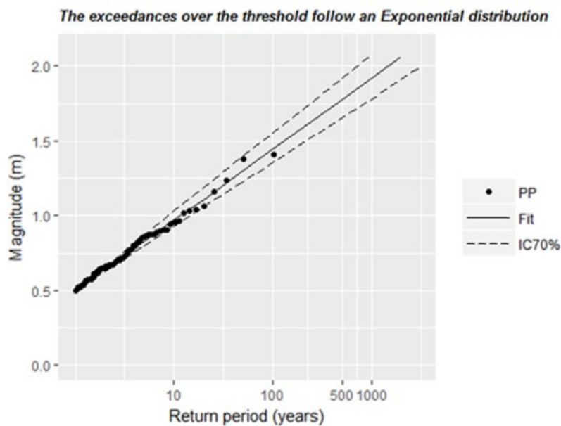
Figure 3.2. Fitting of the SM-Case1 data sets (w=100 years) with GPD distribution
