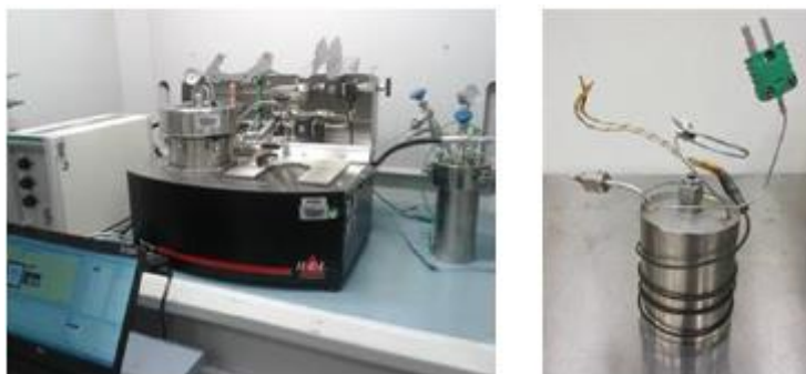
Figure 2: Phi-Tec II calorimeter and its external reactor (left), reaction cell (right)
